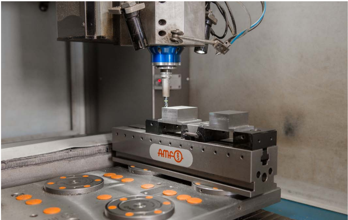
AMF multiple clamping system in conjunction with the AMF zero-point system.
