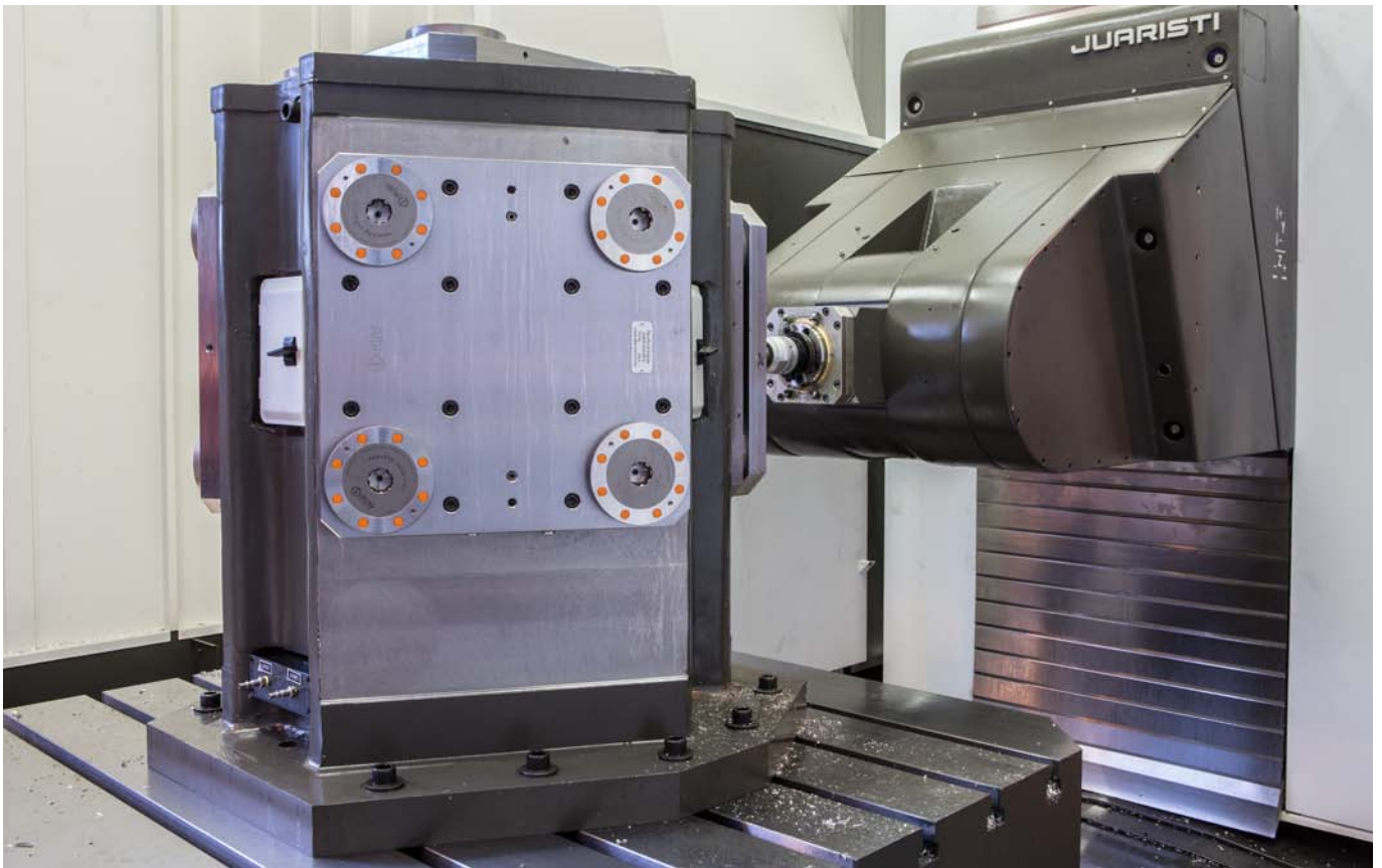
Clamping profile with three pneumatic 4-point clamping stations. Thanks to the high pull-in forces of the zero-point system, changing the clamping device becomes simple and user friendly even in the case of horizontal applications.
