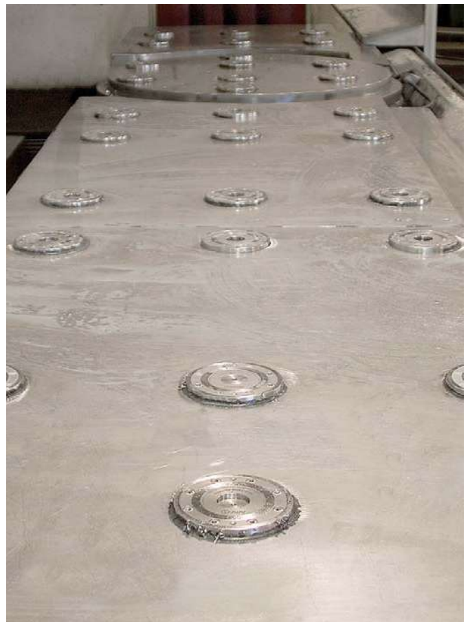
The cylindrical design of the pull-studs and the adapter in the clamping module guarantee a balance of height and length tolerances even at long distances.
