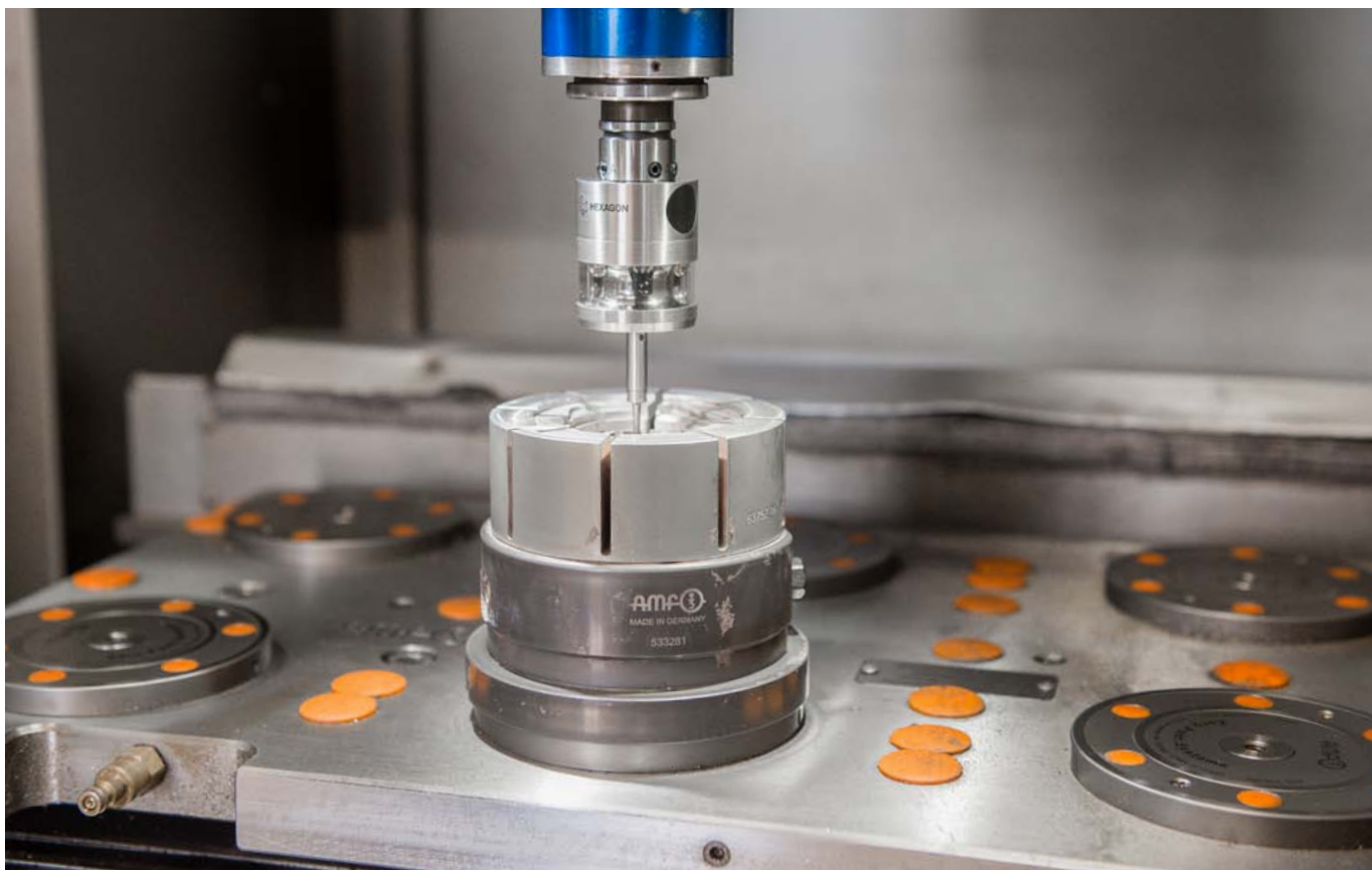
The mechanical collet is clamped directly using zero-point clamping technology. Ideal for clamping thin-walled or sensitive workpieces with complex outer contours.
